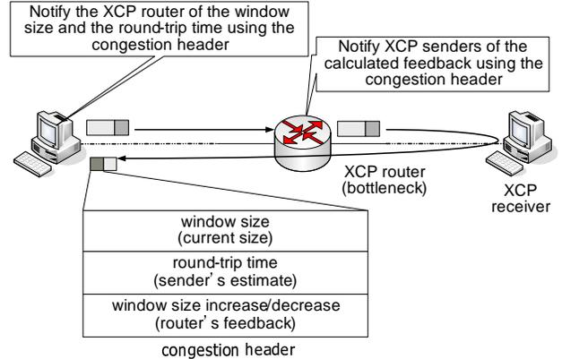
Fig. 1: Overview of XCP congestion control using congestion header
