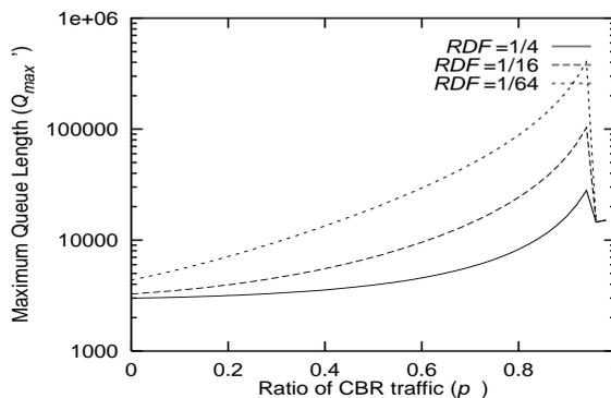
Figure 12: The Maximum Queue Length vs. Ratio of CBR Traffic for  $RIF = 1/1024$  and  $C_{RM} = 32$ .
