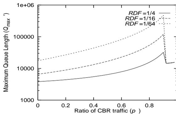
Figure 11: The Maximum Queue Length vs. Ratio of CBR Traffic for  $RIF = 1/64$  and  $C_{RM} = 32$ .
