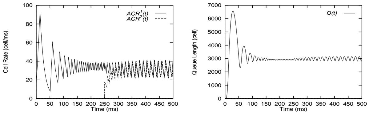
Figure 6: Effect of Propagation Delay for  $\tau_1 = 0.02$  ms and  $\tau_2 = 2.00$  ms.
