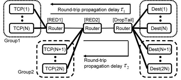
**Figure 2. Network model: case of multiple TCP connections traversing different numbers of RED routers**
