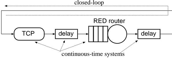
**Figure 1. Modeling entire network by interconnecting continuous-time systems**
