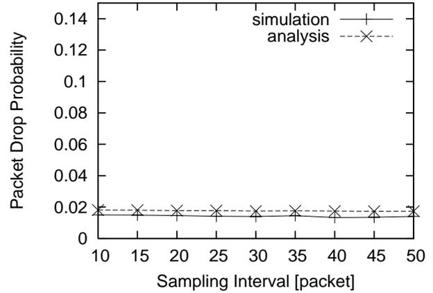
**Figure 4.** Packet drop probability of DRED in steady state (sampling interval  $\Delta t = 10 - 50$  [packet])
