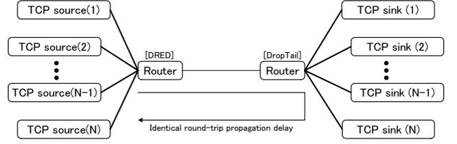
Figure 2. Network topology used in numerical example and simulation
