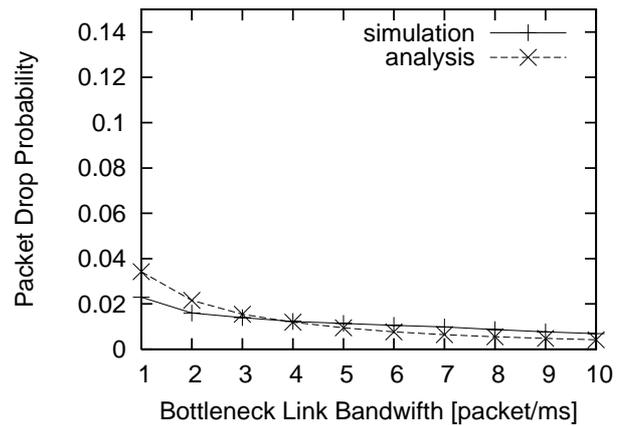
**Figure 8.** Packet drop probability of DRED in steady state (bottleneck link bandwidth  $\mu = 1 - 10$ )
