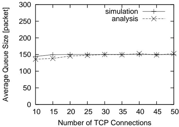
**Figure 5.** Average queue length of DRED in steady state (number of TCP connections  $N = 10 - 50$ )
