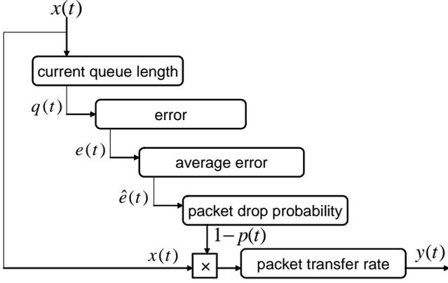
Figure 1. A block diagram for analytical model of DRED
