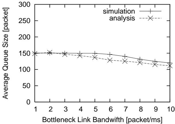
**Figure 7.** Average queue length of DRED in steady state (bottleneck link bandwidth  $\mu = 1 - 10$ )
