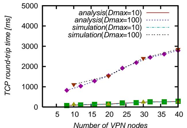
Fig. 6: Number of VPN nodes  $N$  vs. TCP round-trip time  $R_N$ .
