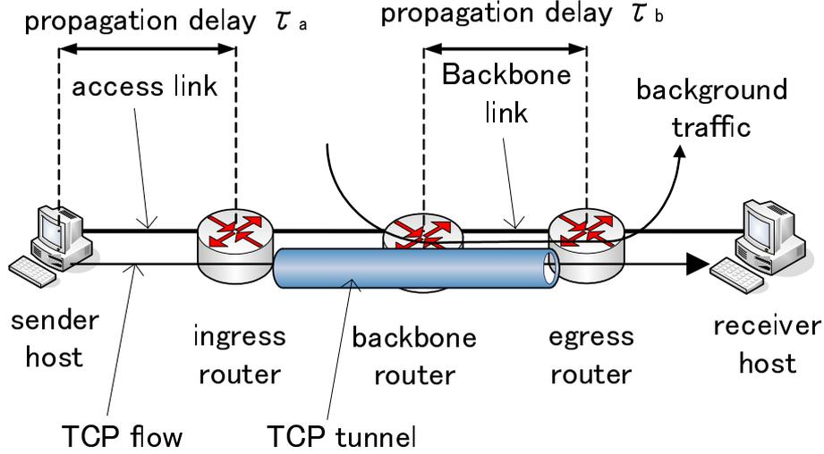
**Figure 1.** Network topology used in simulations
