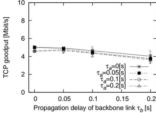
**Figure 2.** TCP goodput with TCP tunnel (effect of propagation delays of access link and backbone link)
